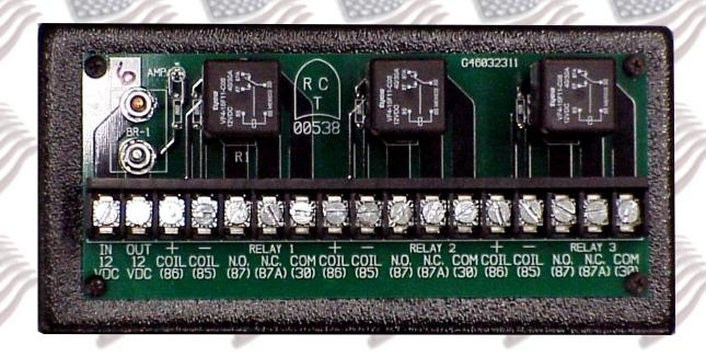
Three Relay PCB, Form C Outputs.
