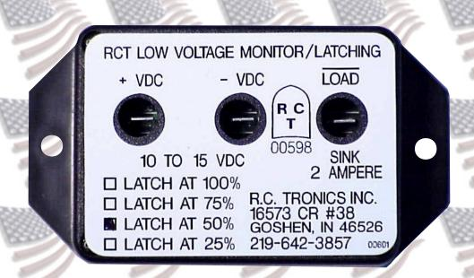
This control is designed to latch to battery negative when voltage level drops below a preset level. It will remain in that condition until power is removed from load.
