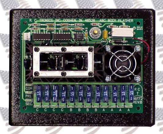
Primary operation; A and C with B 180 degree out of phase. (5 ma. sink)
