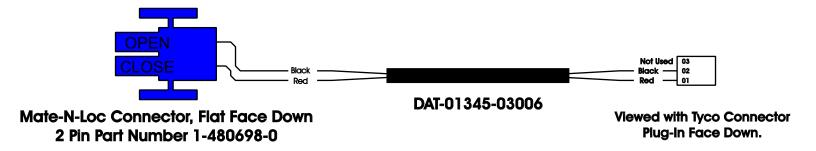
This Data Cable operates Electric Door on Microline Controllers, RCT-01490, RCT-01524, RCT-01507 Interfaces with PCB-01492 and PCB-01493
