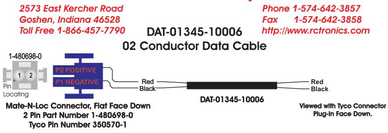
Belden Part Number B-8442 Carol, 22 AWG, Stranded, unshielded two conductor cable. Cut each jacket end 4 inches long, remove jacket on each end. Mate-N-Loc Connector 1-480698-0 Flat face down and insert pins as shown.
