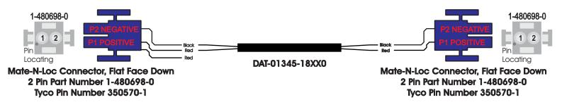
Belden Part Number B-8442 Carol, 22 AWG, Stranded, unshielded two conductor cable. Cut each jacket end 4 inches long, remove jacket on each end. Add heatshrink with DAT part number.
