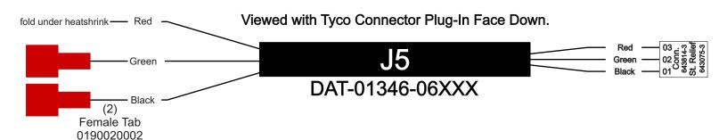
Carol C-4062, 22 AWG, Stranded, unshielded three conductor cable. Cut each jacket end 4 inches long, remove jacket on each end. Add heatshrink with DAT part number.
