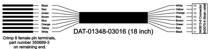
Carol C-2465, 22 AWG, Stranded 7/30/8, unshielded eight conductor cable. Cut each jacket end 4 inches long, remove jacket on each end. Place connector into insertion equipment, start with #8 and complete with #1 Requires one (1) Tyco/Amp. 643813-8 connector & Tyco/Amp. 643075-8 end cap.
