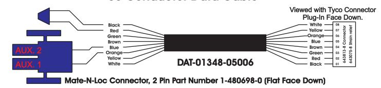
Tyco Connecor Operates Relays 5A & 5B on RCT-00786 or RCT-01414, Bus Power Center from J3 on RCT-00948, Dash Switch Center. Black & Red Operates 7A & 7B when taken to an external ground, with "IGNITION".
