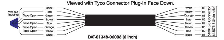
Operates Relays; 6A, 7A & 7B on RCT-00786 or RCT-01414, Bus Power Center from J3 on RCT-00948, Dash Switch Center with "IGNIION"
