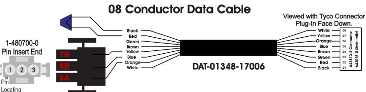
Mate-N-Loc Connector, 3 Pin Part Number 1-480700-0 (Flat Face Down)
