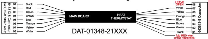
Carol C-2465, 22 AWG, Stranded 7/30/8, unshielded eight conductor cable. Cut each jacket end 4 inches long, remove jacket on each end. Add heatshrink with DAT part number.
