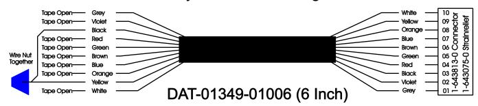
Enables "Emergency Master" for RCT-00786 or RCT-01414, Bus Power Center from J4 on RCT-01069, Dash Switch Center. When Switch #12 is not used.
