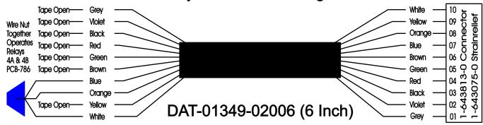
Operates Relays 4A and 4B with "IGNITION", on RCT-00786 or RCT-01414, Bus Power Center. Connects to J4-PCB-01083.
