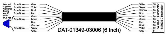
Operates Relays 4A, 4B and 5B with "IGNITION", on RCT-00786 or RCT-01414, Bus Power Center. Connects to J4-PCB-01083.
