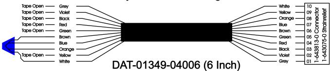
Operates Relays 4A, 4B and 5A with "IGNITION", on RCT-00786 or RCT-01414, Bus Power Center. Connects to J4-PCB-01083.
