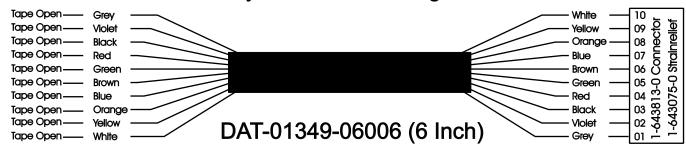
Carol C-9540, 24 AWG, Stranded 7/32/10, Foil 24 AWG Gnd shielded ten conductor cable. Cut each jacket end 4 inches long, remove jacket on each end. Requires one (1) Tyco/Amp. 1-643814-0 connector & Tyco/Amp. 1-643075-0 end cap. Place connector into insertion equipment, start with #10 and complete with #1
