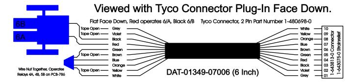
Mate-N-Loc operates relays 6A & 6B with "IGNITION", on RCT-00786 or RCT-01414, Bus Power Center connects to J4 on RCT-01083, Dash Switch Center.
