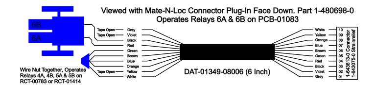
Mate-N-Loc connector operates relays 6A & 6B with "IGNITION, on RCT-00786 or RCT-01414 Bus Power Center. Connects to J4 on RCT-01083 Dash Switch Center.
