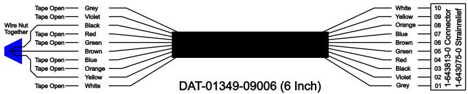
Operates Relay "6B" and Enables "Master Switch" with "IGNITION", on RCT-00786 or RCT-01414 Bus Power Center from J4 on RCT-01069, Dash Switch Center.
