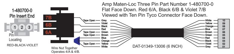
Mate-N-Loc operates relays 6A, 6B & 7B with "IGNITION", on RCT-00786 or RCT-01414, Bus Power Center connects to J4 on RCT-01083, Dash Switch Center.
