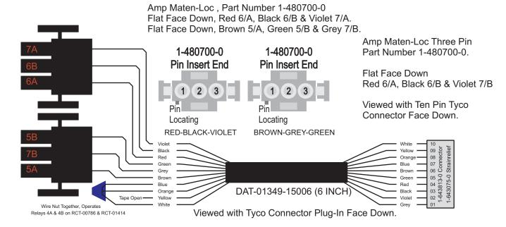
Mate-N-Loc's operates relays 6A, 6B, 7A & 5A, 5B, 7B with "IGNITION", on RCT-00786, RCT-01414 and RCT-01760, Bus Power Center's. Connects to J4 on RCT-01083, Dash Switch Center. Blue, Orange and White Operates 4A, 4B, with "IGNITION".
