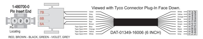
Mate-N-Loc operates relays 7B, 7A - 6B, 5B- 6A, 5A on RCT-00786 or RCT-01414,
