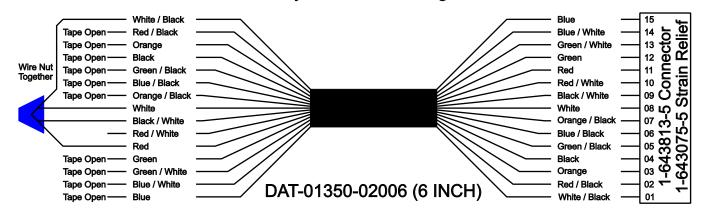
Operates Relays; 4A, 4B and 5B with "IGNITION" on RCT-00786 or RCT-01414. Bus Power Center. Connects to J3-PCB-01067 or J1-PCB-01068.
