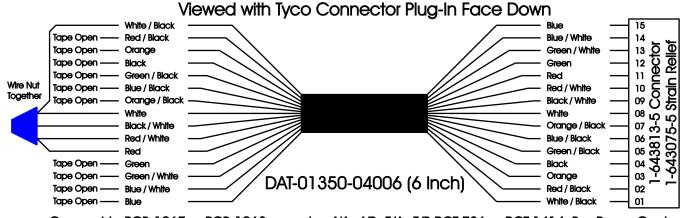
Connect to PCB-1067 or PCB-1068 operates 4/A, 4/B, 5/A, 5/B RCT-786 or RCT-1414, Bus Power Center
