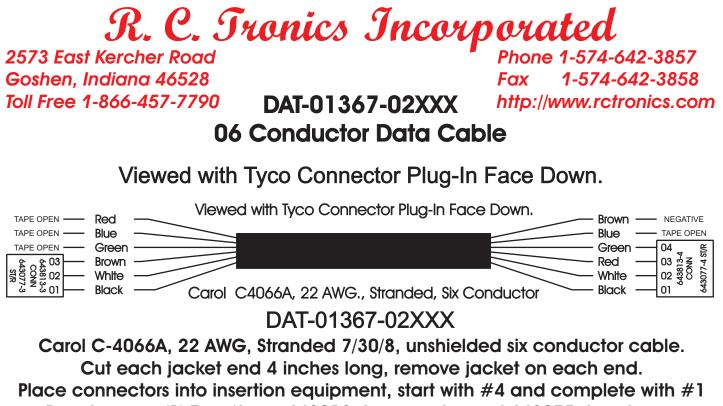
Requires one (1) Tyco/Amp. 64381<u>3</u>-4 connector and 643075-4 end cap. Also add (1) Tyco/Amp 64313-3 connector & (1) 643075-3, begin with #3 and end with #1.
