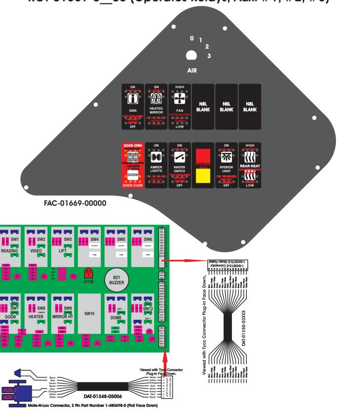
Tyco Connecor Operates Relays 5A & 5B on RCT-00786 or RCT-01414, Bus Power Center from J3 on RCT-00948, Dash Switch Center. Black & Red Operates 7A & 7B when taken to an external ground, with "IGNITION".
