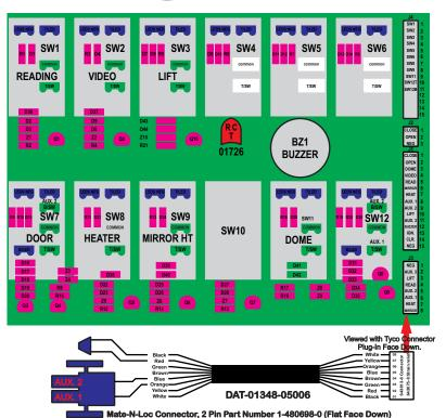
Tyco Connecor Operates Relays 5A & 5B on RCT-00786 or RCT-01414, Bus Power Center from J3 on RCT-00948, Dash Switch Center. Black & Red Operates 7A & 7B when taken to an external ground, with "IGNITION".
