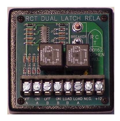
System will control two loads with momentary switches. Will operate loads from multiple locations.
