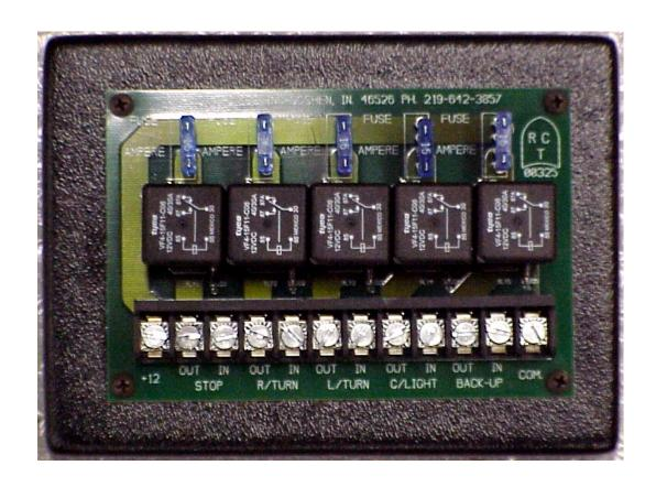
Five Relay with Relay On LEDs.
