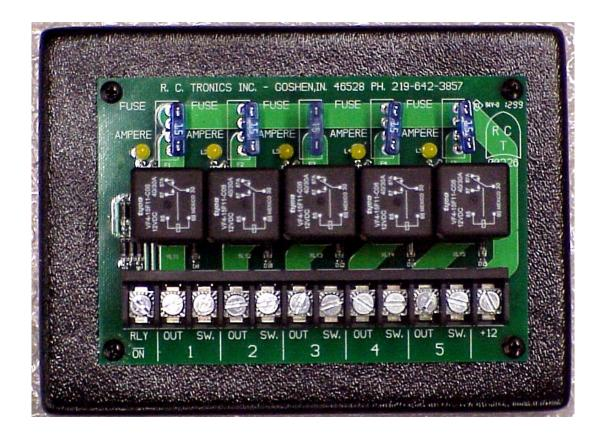
Five Relay with Relay On LEDs.
