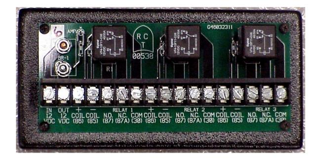
Three Relay PCB, Form C Outputs.
