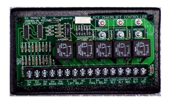
SW. ON-----Normally connected to switch, which operates to Battery Negative, Enables RCT-540.
