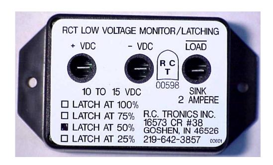
This control is designed to latch to battery negative when voltage level drops below a preset level. It will remain in that condition until power is removed from load.
