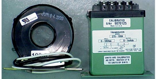
Current Transducer. One Required For Each Current Meter Pin #1 of Current Meter, (red) to +12 VDC Pin #2 of Current Meter, (black) to - VDC (common) Pin #3 of Current Meter, Not Used Pin #4 of Current Meter, Not Used Pin #5 of Current Meter, (green) to Current Transducer Terminal #2 Pin #6 of Current Meter, (white) to Current Transducer Terminal #1
