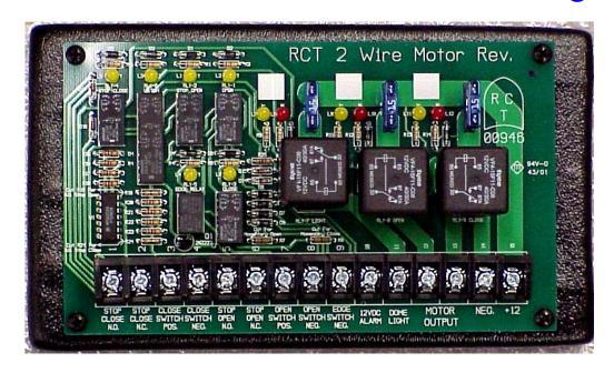
Control can be used with both momentary or maintained, "Command Open or Closed' switchs. These inputs can be positive or negative.
