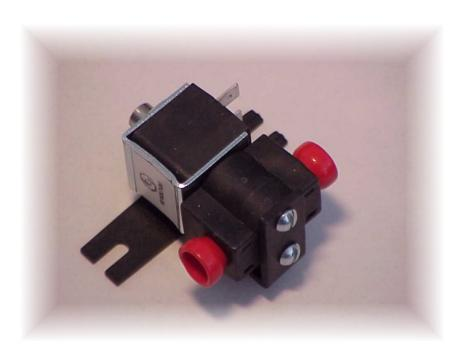
This is a twelve volt d.c., 24 watt, 3-way N.C. solenoid valve. Coil Class A (105 deg. C). Operating temperature 120 degree F. Valve body is Polypropylene, seals NBR with a body orifice of .062. Electrical Connection via two .250 male tabs. Unit requires mounting area of two and three fourths inches with a depth of two inches.
